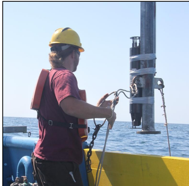
Figure 2.2: In situ deployment of LISST-100X particle size analyzer at R/V Brooks McCall.
