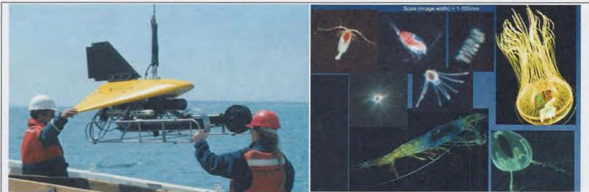
Fig. 1 Digital Automatic Video Plankton Recorder (DAVPR). (left) DAVPR being deployed, (right) example images from the DAVPR (image widths range from 1- 100mm)
