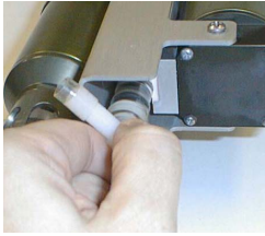
Rotate C Duct clockwise
