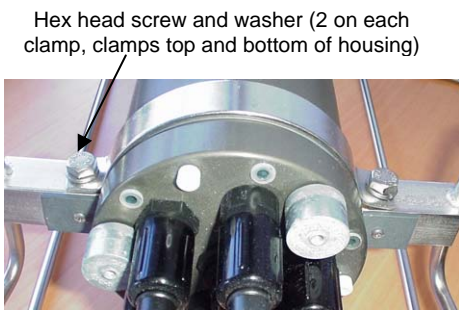
Remove plastic hex-head screw (typical, 3 places)
