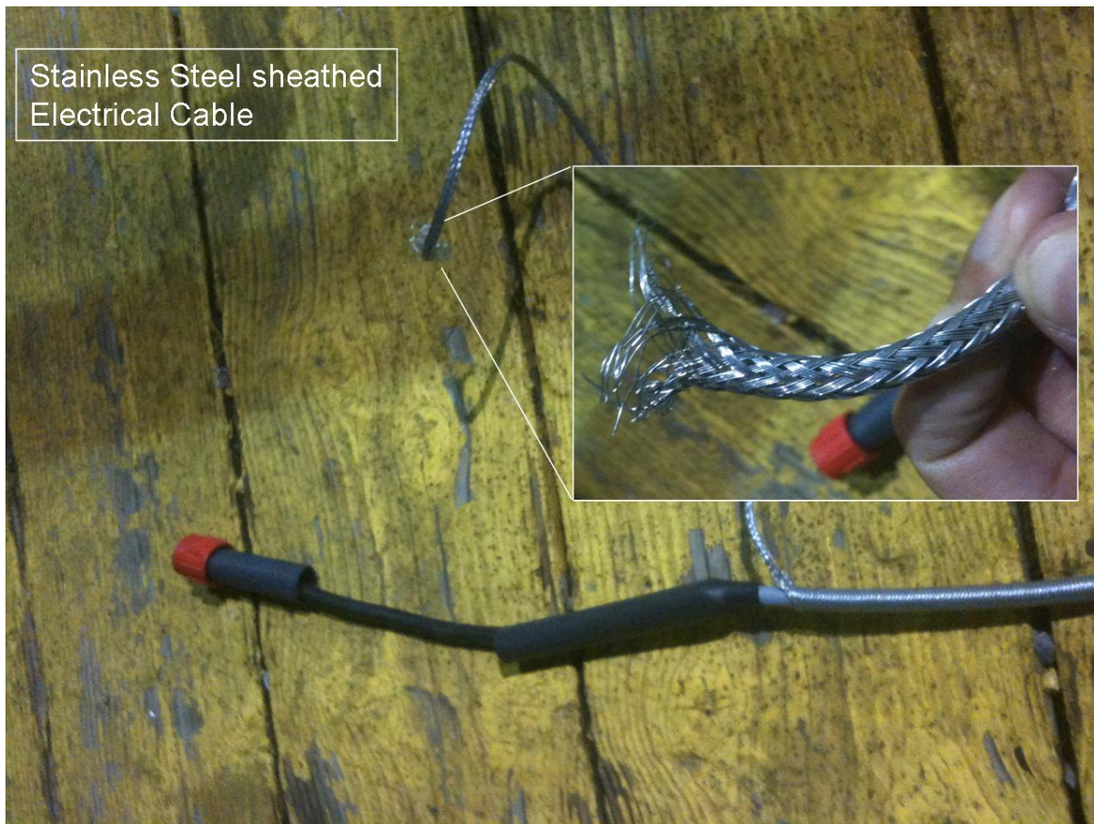
Photograph 11. New electrical cable sheathed in stainless steel wire for 150m pump hose. The steel weaved mesh will support over 800lbs of weight.
