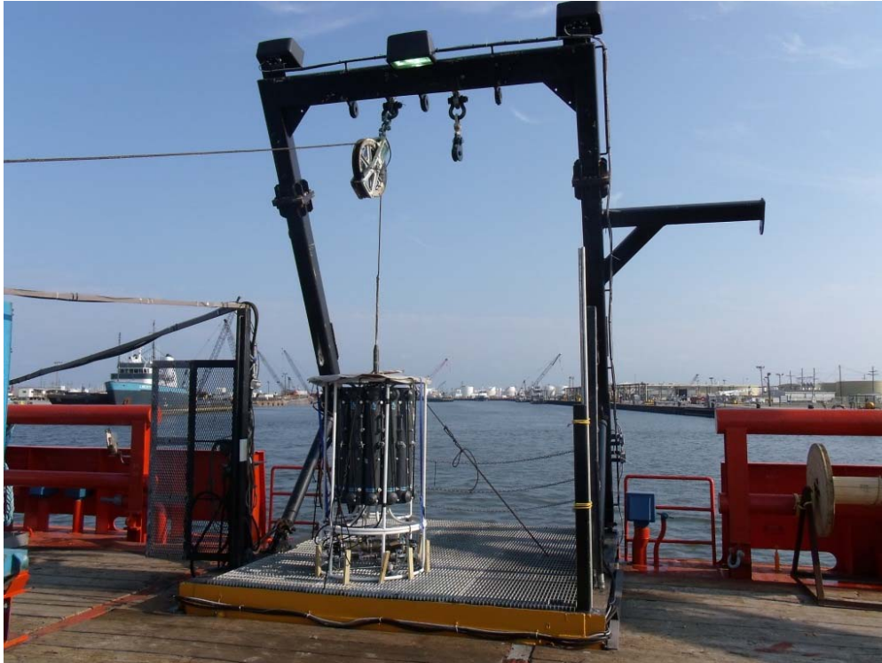
Photo 1. CTD Rosette deployment deck and A-frame
