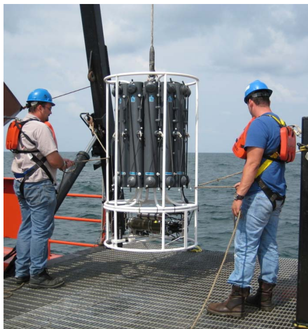
Figure 4 – CTD / rosette array being deployed by C&C technicians.
