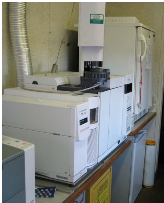
Figure 7 – GC/MS (Gas Chromatograph/ Mass Spectrometer) capable of identifying PAH compounds in concentrations as low as 10ppb.
