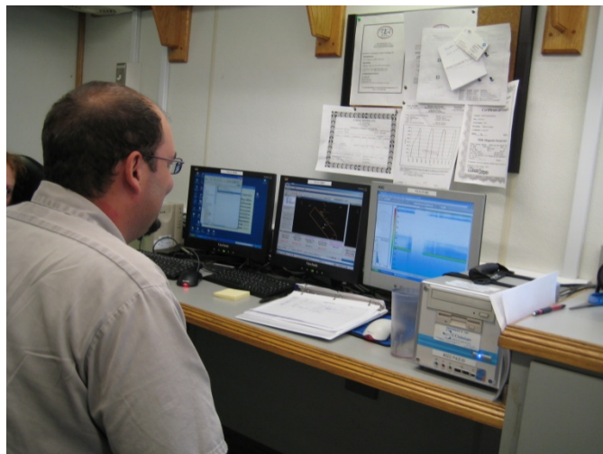
Figure 3 – Sonar acquisition station for the Simrad EK-60 split-beam echosounder. The station allowed surveyors to identify potential hydrocarbon seeps in the seafloor for investigation with the CTD sensor package described below.
