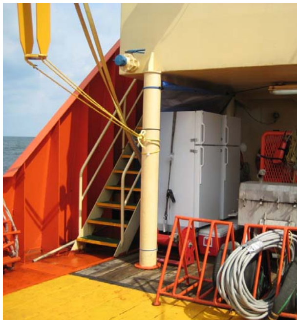
Figure 2 – New water sample refrigerators installed on newly fabricated platform.
