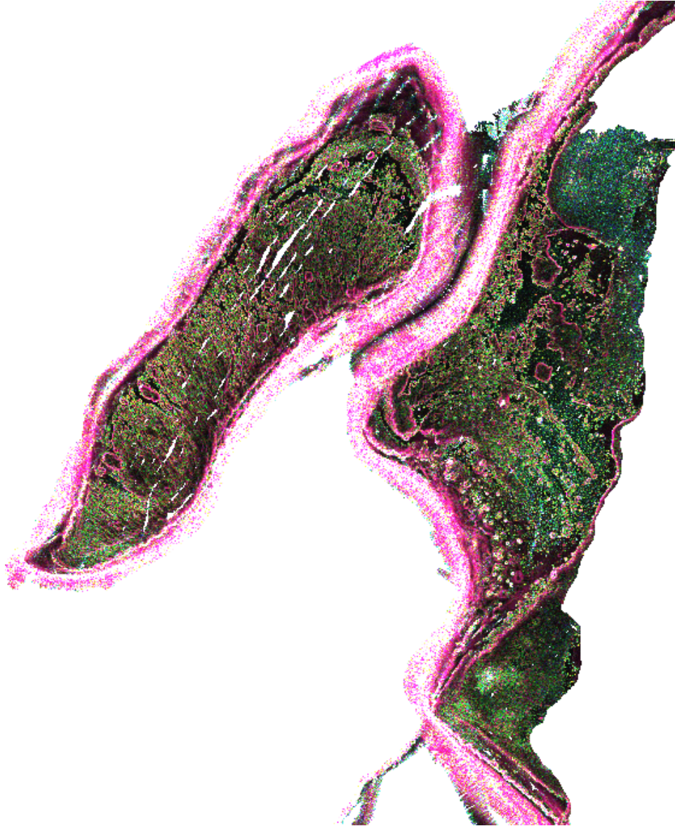
Figure 6. Pseudospectral LFMRGB map for Saipan bathymetry grid with 5 m cellsize. Red Green and Blue image color band values represent weighted values of local Fourier coefficients 1, 2, and 3 ( F(1) , F(2) , F(3) ), which represent variation at a range of spatial frequencies relatively low, medium, and high.
