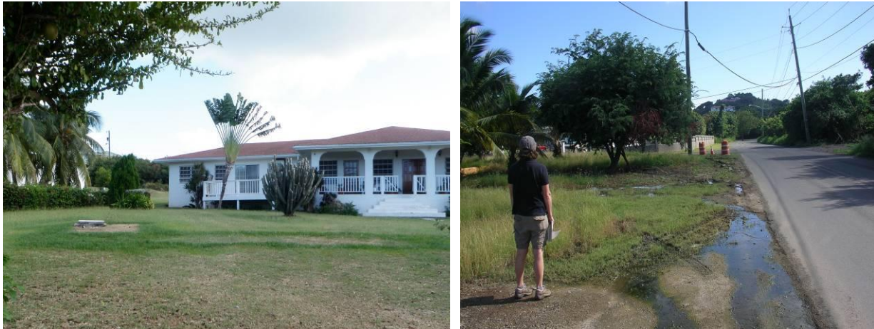
Figure 3.8. Green rectangular indicators of septic system on single family lot (left). Record high groundwater tables and resulting surface seepage in Tipperary/All for the Better residential areas may have resulted in failing septic systems (right).
