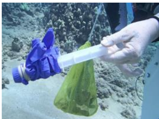
Figure 17. Sediment collection using a modified syringe technique and capping with nitrile gloves.
