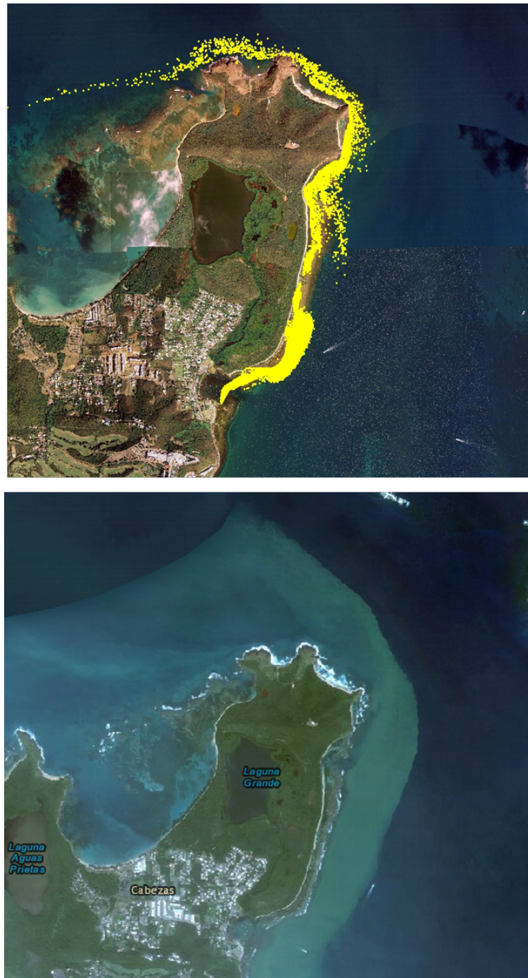
Figure 4.18: Visual comparison between computed particle positions and an aerial picture from Google Earth showing a suspended sediment plume.
