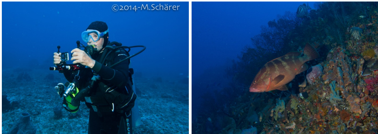
Figure 3. Video and laser caliper method at left (photo by M. Schärer) and lights from red laser on Nassau grouper at right (photo by H. J. Ruiz).
