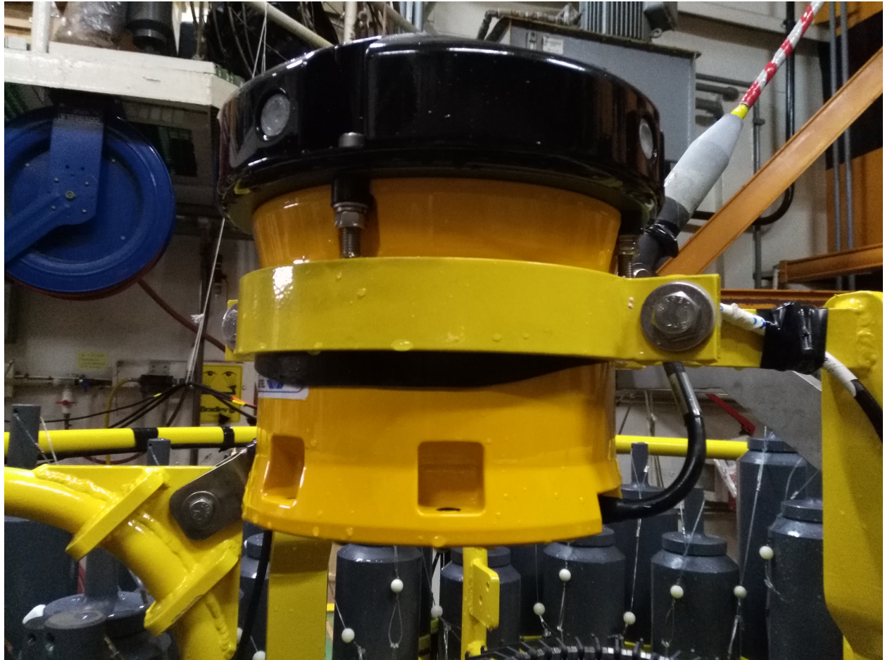
Fig. 17.2: Upward looking ADCP
