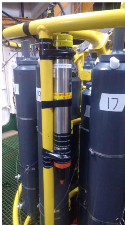
Fig. 18.1: Chipod pressure case attached on the rosette
